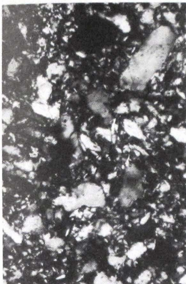
4. Sample of clay core material magnified 200 times, with quartz and feldspar grains showing typical subrounded edges common in sediments that have been transported along a river-bed (in crossed polarized light).
