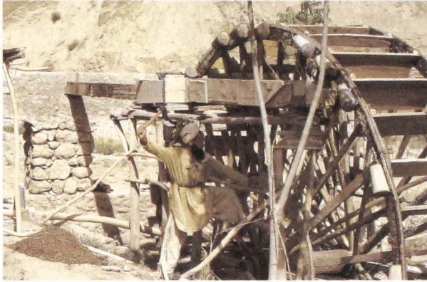
Details of water wheel showing paddles that propel wheel, lifting perimeter buckets of water from a river for distribution through juis to fields.
